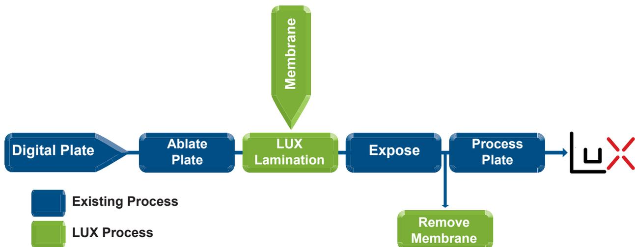
The LUX Laminator is a simple addition to your existing digital workflow. LUX Membrane 100 is laminated to the digital plate following laser ablation. This lamination process takes between 4-6 minutes, and works with all plates, including the largest available size, 52" x 80" (1321 mm x 2032 mm). Following exposure on your existing unit, the Membrane is peeled off and disposed in seconds. The plate can then be processed in your existing equipment.
